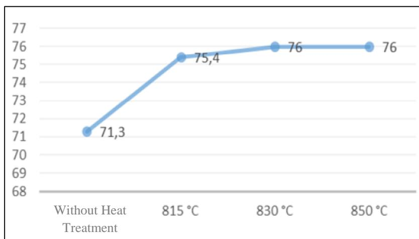
Picture 5. Graph of Total Results Average Hardness Test
