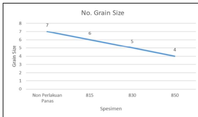
Picture 3. Graph of Microstructure Grain Calculation Results
