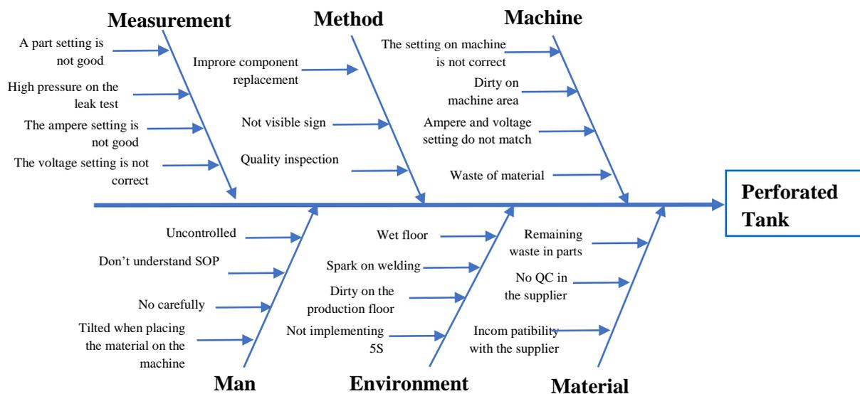
Figure 6. Fishbone diagram of perforated tank
