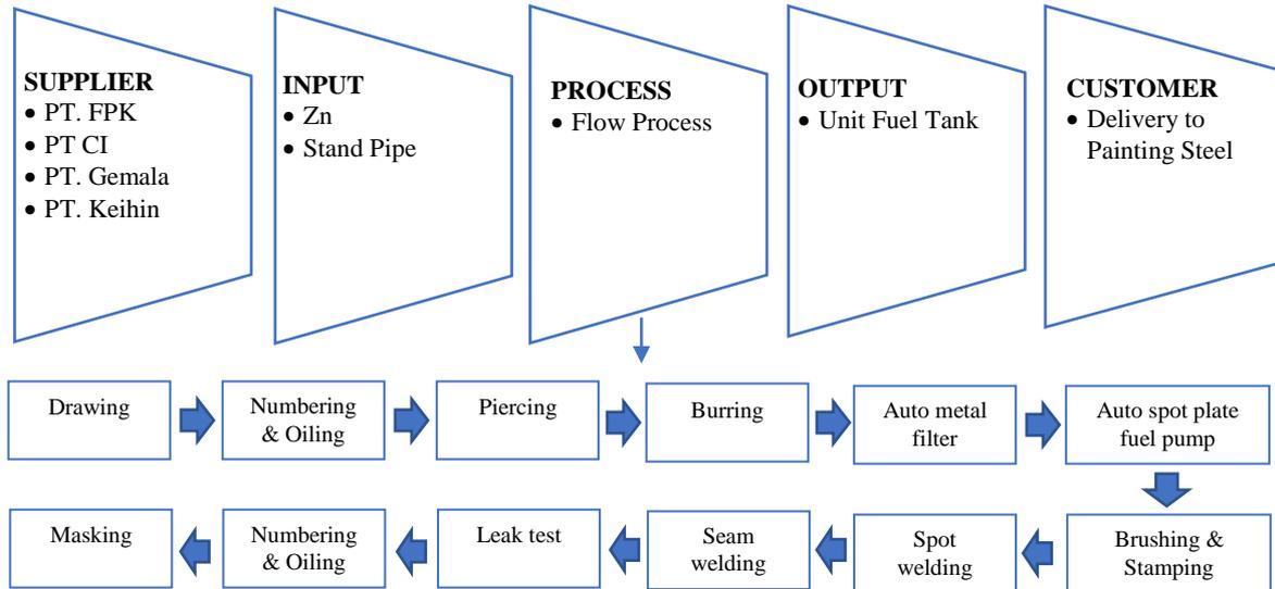
Figure 3. SIPOC diagram of production flow
