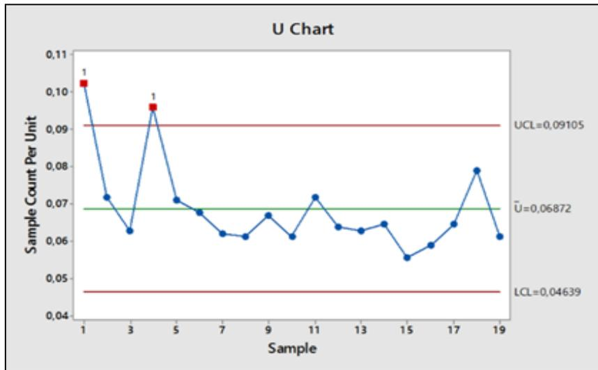
Figure 5. U-Chart of sample defect
