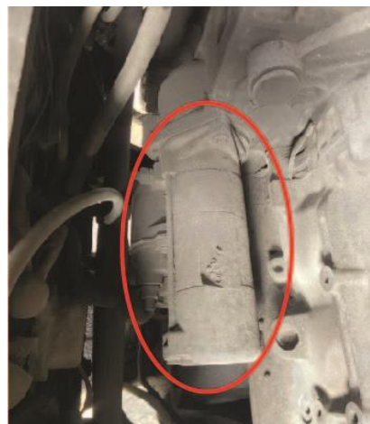
Figure 2. Starter Dynamo Spare-part Source: Mechanical Maintenance
