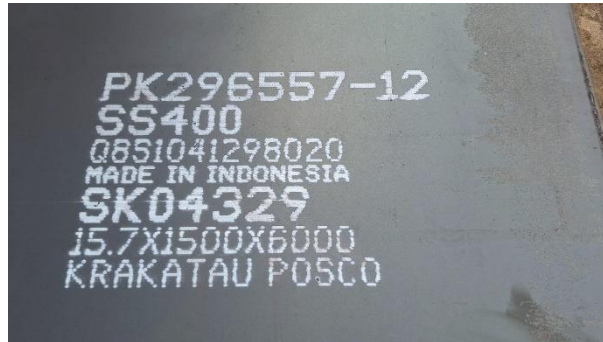
Figure 4. SS400 steel material with a thickness of 16 mm
