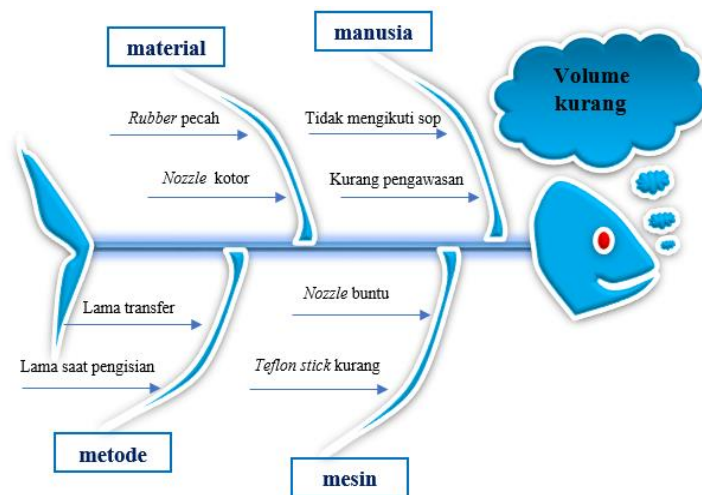
Figure 9. Cause and Effect Diagram of Low Volume Defects
