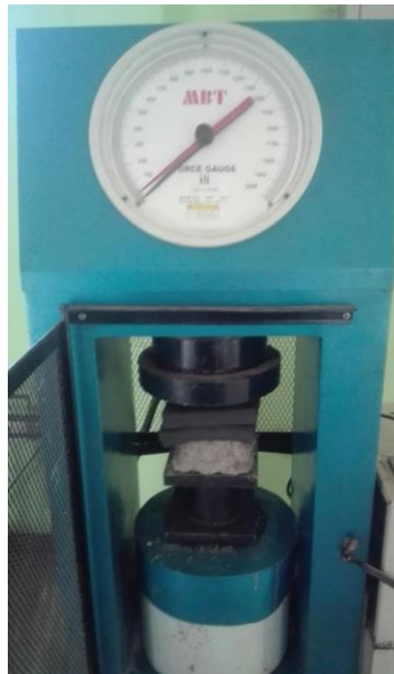
Gambar 12. Hidrolic compression concrete beam
